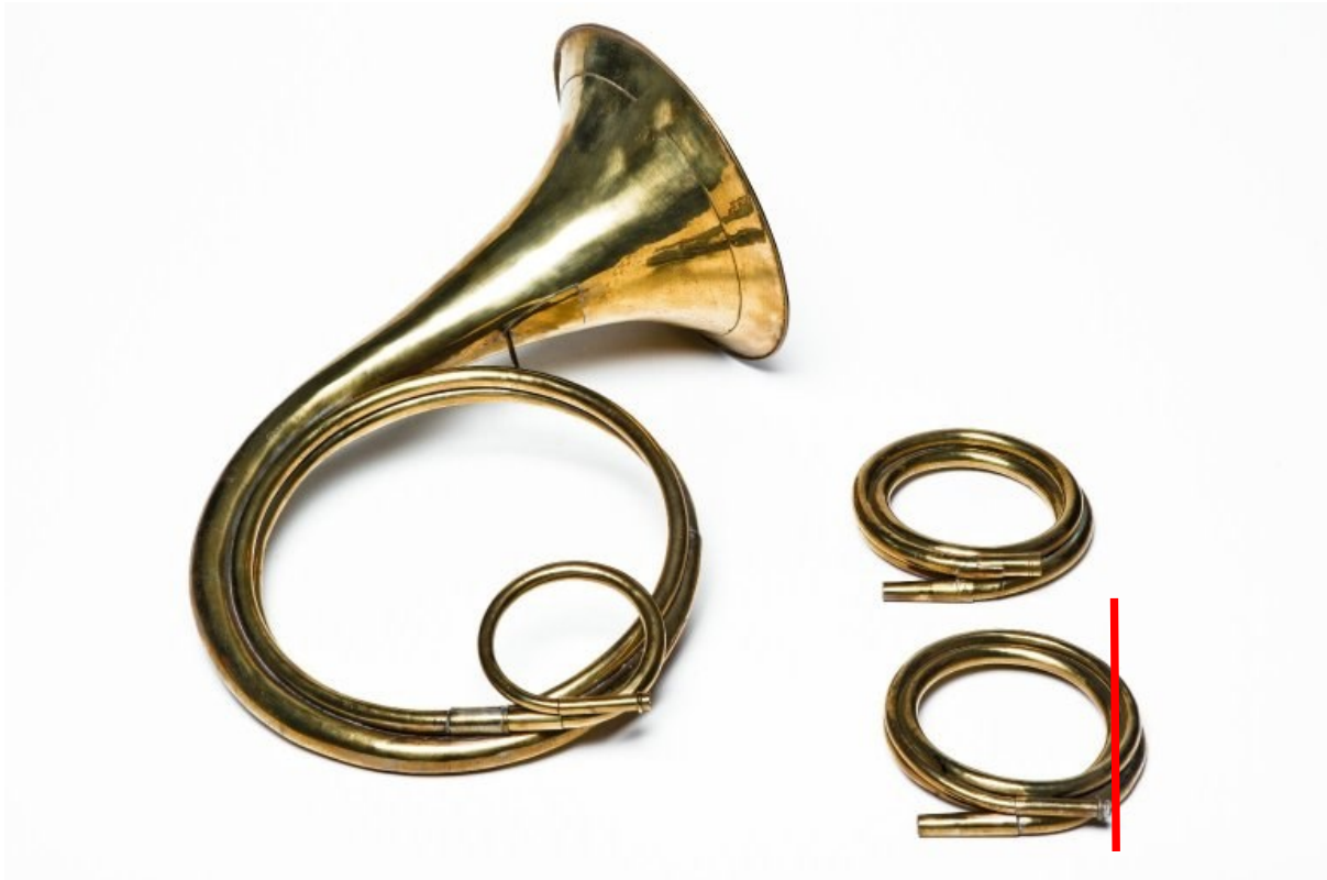
Fig. 3: Instrument 2888 with a master crook and an additional master crook and coupler. The red line shows that it is not possible to correctly insert the instrument into the flat measuring head. ( http://www.mimo-db.eu/UEDIN/2888 )
